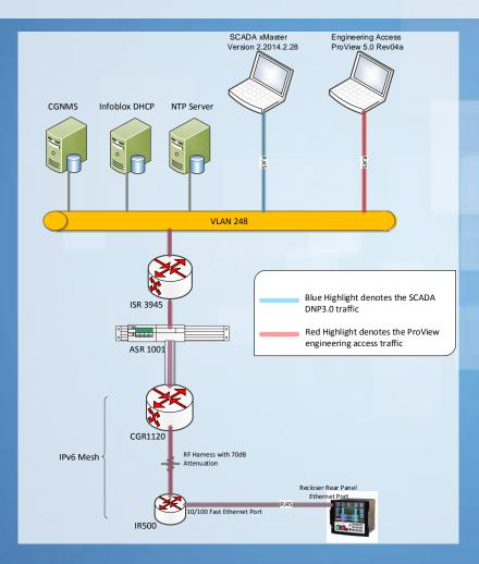
Conversion of IPv4 to IPv6 was necessary for the Distribution Automation devices to work.
