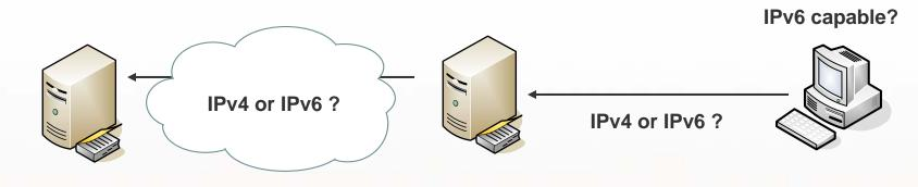
The lookup of A versus AAAA records is independent of whether the DNS packets are carried over IPv4 or IPv6
